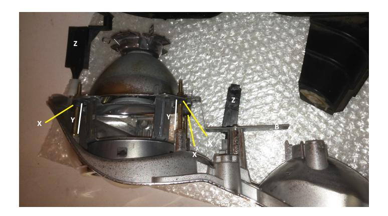
When you bolt the projector unit back onto the frame, make sure you do NOT squeeze the rubber sleeves (X) too hard. They take up vibrations, and therefore should just start to compress. Also check that they tightened the same distance (Y) from the lower nut (measure).
