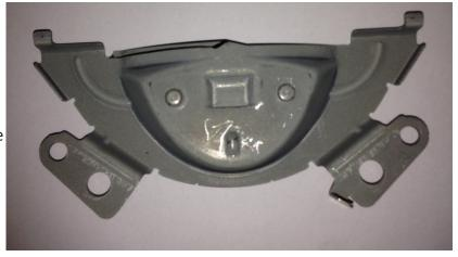
Next you find a suitable piece of bendable metal e.g. aluminium (<1 mm thick), which you cut to size (35 x 7 mm) and bend along the backside of the harmonizer, then file to match (mirror) the profile you filed off. Glue it on with epoxy type glue or similar.
